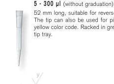
52 mm long, suitable for reverse pipetting. The tip can also be used for pipettes with yellow color code. Racked in green-colored tip tray.
